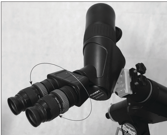
Figure 4. The BinoViewer swivels 360 degrees to allow positioning of the two eyepieces at a comfortable viewing angle.
